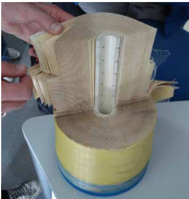
Reverse osmosis membrane cut open
